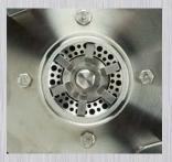
shearing action and "pre-mixes" the materials prior to entering the secondary stage. Particle and droplet size reduction down to 5 - 7 microns is typical in this stage.
