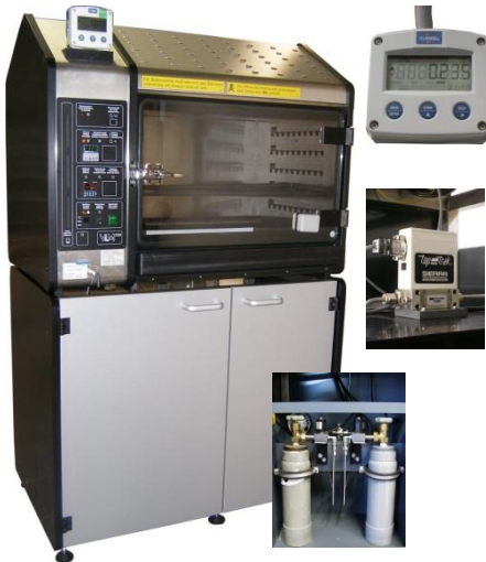
Figure 4 CON 300-FL with electronic dosing system for SO 2
