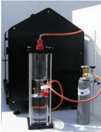
Figure 3 Manual dosing system for SO 2
