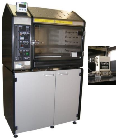
CON 300-FL with electronic dosing system DosiCORR® ED
