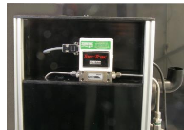
Casket with the SO 2 bottle and the electronic mass flow meter
